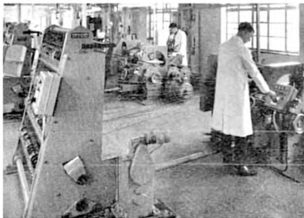
Left: The tape-coating machine, and (right) the tape-slitting process
